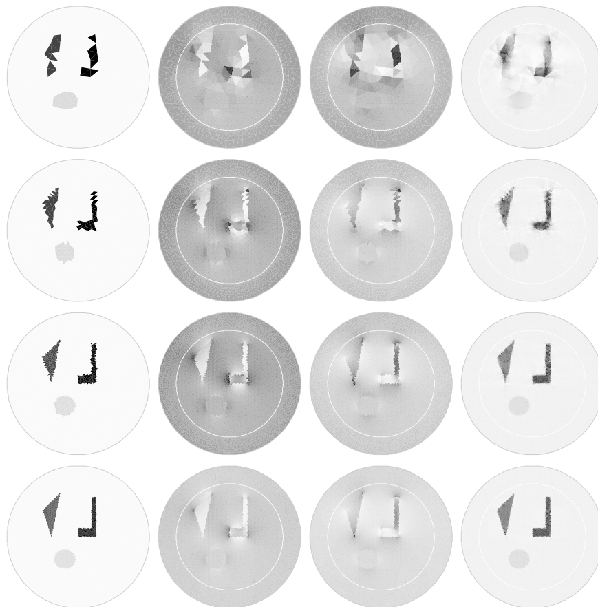
FIGURE 4.4. Reconstruction tests. From top to bottom, using a regular mesh with 50,100,200, and 400 boundary points. From left to right, the initial guess, the collected data \mathcal{S} (for x/|x| and y/|y| ) and the reconstructed conductivity.
