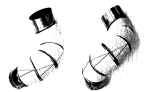
FIG. 2. Variable model construction of two 3-inch (7.62 cm) and 4-inch pipe elbows joined to produce a 4-jointed structure. Each cylindrical section is assumed to be 19.3 cm long to the centerline graph paper. The solid line indicates the long axis of each cylindrical section. The dashed line represents the "B" belt angle. The structure is twisted into a right-hand helix with dimensions approximating those of Fig. 1.
